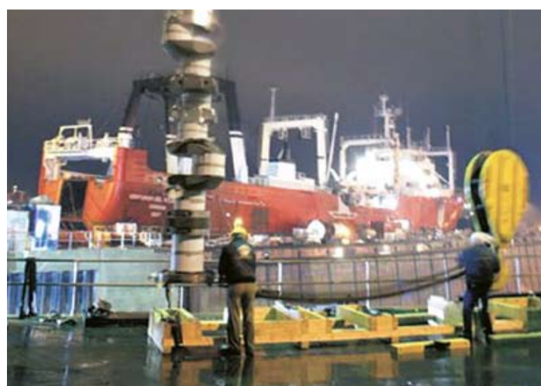
The reconditioned crankshaft pictured on its restoration to the engine room
