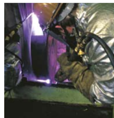
The bulkhead between the engine room and first cargo hold was cut open to create extra space for, among other things, the propane gas canisters and burners used in heating up the crank web
