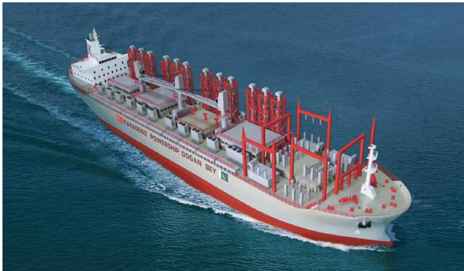
Illustration of a 'power ship'. Freighters will be converted into floating diesel power plants that can be connected to local power grids to temporarily cover demands whenever onsite power plants are insufficient or new power plants cannot be built quickly enough. Unlike so-called 'power barges' – power plants on pontoons – the power ships will be capable of self-propulsion
