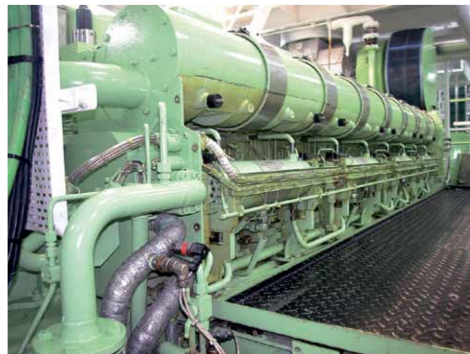
The tuna-freezing purse seiner is powered by an MAN 8L32/44CR medium-speed main engine
