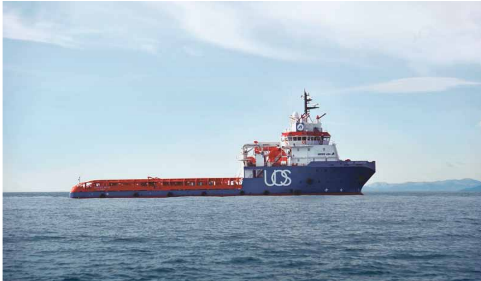
The Hartmann tug "UOS Atlantis"; like the other five tugs covered by the agreement, its four 6L32/40 engines produce an impressive 180 ttp (tons bollard pull)
