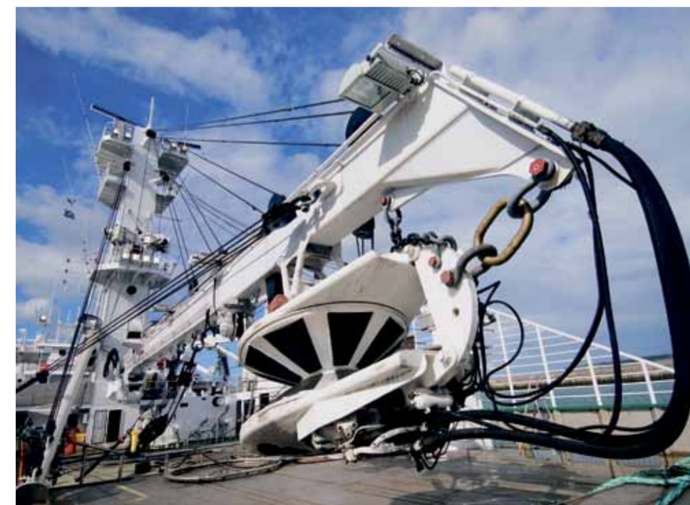
Hydraulic crane aboard the Playa de Azkorri
